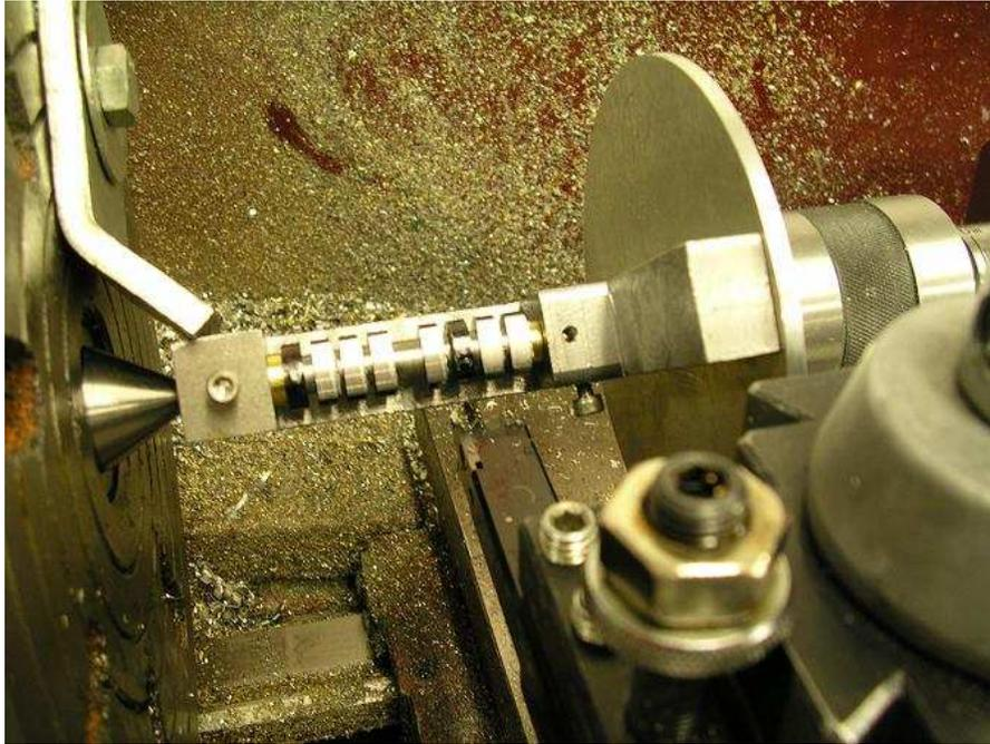
Repeat this process until the cam has made a 180 degree swing in 5 degree steps. If this is done correctly, the pointer should be pointing to 90 degrees.
