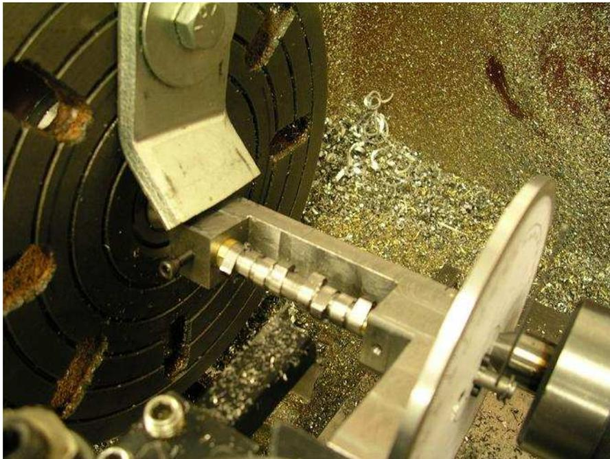
Remove the shaft from the fixture and chuck it up so you can use the lathe to hold the piece. Using a small file I round the nose of the lobe over. After all the filing is done, I take a piece of sand paper and polish the file marks out by running the lathe forward and holding the paper to each lobe. Then repeat the process with the lathe turning in reverse to polish the other side of the lobe.
