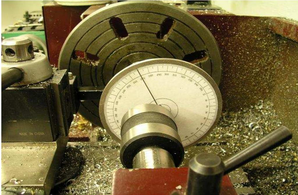
I made all my cuts in .005 deep steps. I felt the extra time was worth spending rather than taking a chance of the shaft spinning in the fixture unexpectedly. I also used a carbide insert type tool and they do not like the constant hammering of an interrupted cut. I was able to complete all the cuts without an insert change increasing my chances of a consistent lobe shape.
